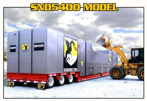
The SND5400 is a 54 million BTU/hr machine and is rated at melting 180 tons of snow per hour (600-1800 cubic yards of snow per hour) - based on the Latent Heat of ICE. Since every manufacturer uses a different ton rating, you must compare snowmelters by their BTU's, as a result this snowmelter is comparable to 350 ton melters being sold in the marketplace. This model can be supplied as a mobile or stationary melter and will operate on diesel fuel, Jet A fuel, propane, or natural gas.
