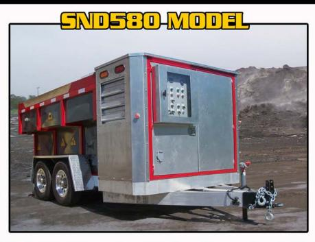
The SND580 is a 5.8 million BTU/hr machine rated at melting 18 tons/hour - Based on the Latent Heat of Ice. Since every manufacturer uses a different ton rating calculation, you must compare snowmelters by their BTU's. In comparison, this model is larger than 20 Ton/hr snowmelters being marketed in the industry.
